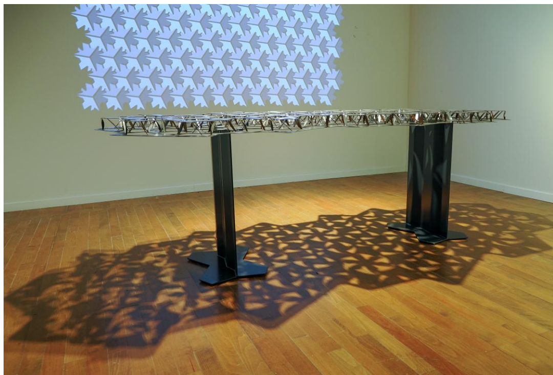
Figure 3: Kirigami space frame sustaining its self-weight between two support points.
