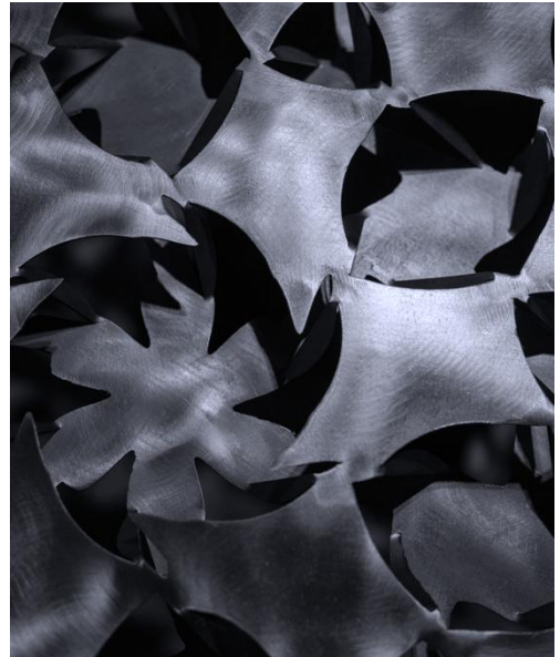
Figure 1: Deployed kirigami space frame with a tiling pattern generated by a continuous normalizing flow.
