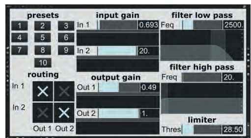
Figure 7: Graphical user interface for the signal processing software. The GUI displays a subset of the control parameters of the digital signal processing
