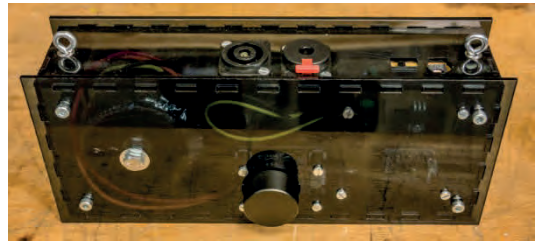
Figure 4: Custom Amplifier. Shown on this photograph is a custom designed amplifier that is used to drive the piezoelectric films as loudspeakers. Visible on the top side of the amplifier are (from left to right): a Speakon socket for connecting the loudspeaker region, a Jack socket for connecting the audio interface, a switch for turning the amplifier on and off, and a barrel socket for connecting a power supply. Visible on the front of the amplifier is the volume control knob. Barely visible through the acrylic surface are (from left to
